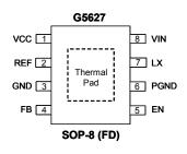
Note: Recommend connecting the Thermal Pad to the GND for excellent power dissipation.
